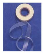
The Ultimate in Armor Protection: Fibertek Res-I-Flex is a B-Staged, epoxy coated, woven polyester/glass tape which shrinks and fuses during the cure cycle to insure a tough, conformal moisture and chemical resistant dielectric seal for AC stators and DC armature coils. During the cure cycle, the resin flows and the polyester yarns in the warp direction shrink providing a leak proof seal and eliminate the need for external pressure to be applied.
